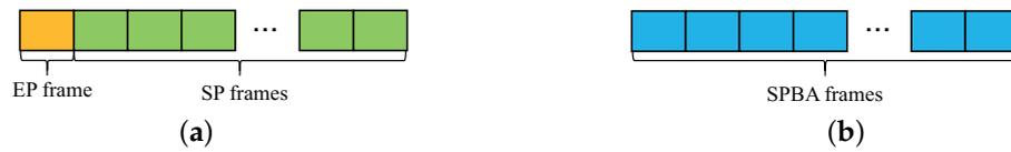
**Figure 2.** The transmitted data frames of (a) SP-OTFS systems and (b) SPBA-OTFS systems.
