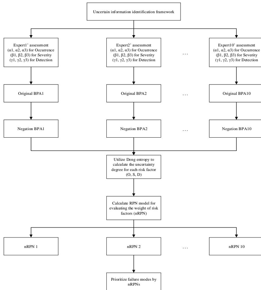
**Figure 1.** The flowchart of measuring the negation information in FMEA with the belief entropy in the DST framework.
