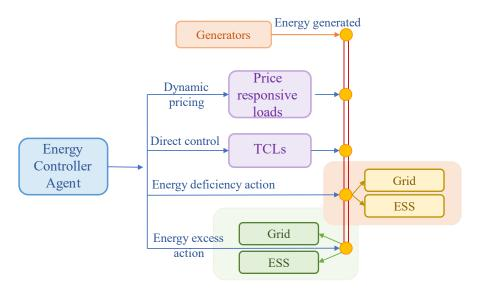
Figure 2. The control mechanism of Energy controller.
