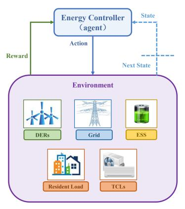
Figure 7. Interaction process between the energy controller and the system environment.
