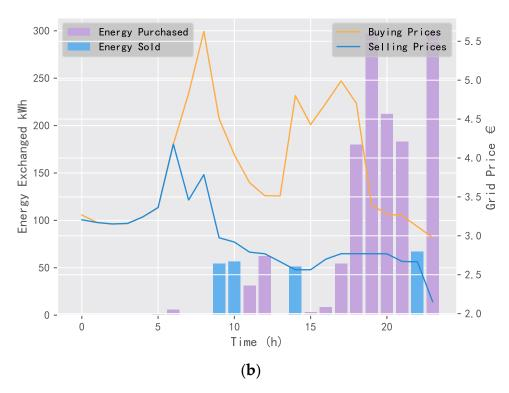
Figure 14. TCLs status and power exchange using DQN: (a) TCLs and (b) power exchange.
