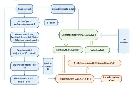
Figure 6. The flow chart of D3QN.
