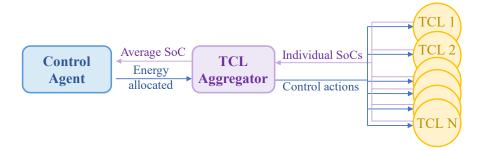
Figure 3. The intermediary role of the TCL aggregator.
