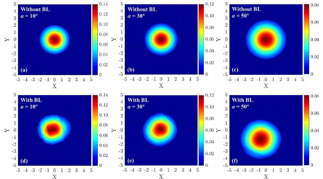
**Figure 9.** The photons distribution probability with different azimuth when the photon via the boundary layer or not. (a–c) show the photons distribution probability of the Gaussian beam without BL. (d–f) show the photons distribution probability of the Gaussian beam that passes through the BL. (a,d) show the situation when the azimuth angle is  $10^\circ$ . (b,e) show the situation that the azimuth angle is  $30^\circ$ . (c,f) show the situation the azimuth angle is  $50^\circ$ .
