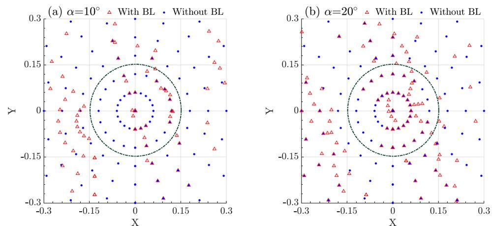
Figure 8. (a) The receiving photons distribution when the azimuth angle is  $10^\circ$  with and without the effect of supersonic BL, which are denoted by a red triangle and blue point respectively. (b) The receiving photons distribution when the azimuth angle is  $20^\circ$  with and without the effect of supersonic BL. The green dotted line indicates the aperture of the receiving telescope.
