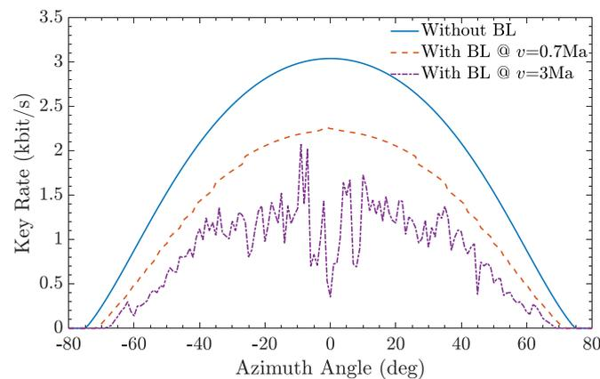
**Figure 10.** The secure key rate over the azimuth angle when the photon via subsonic BL, supersonic BL, or not.
