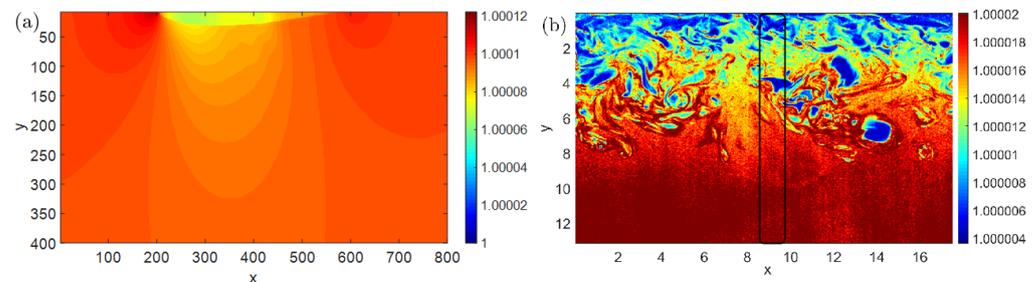
**Figure 3.** The sectional drawing of refractive index field of (a) the airfoil boundary layer and (b) the supersonic boundary layer. The coordinate axis represents the size of the boundary layer, in millimeters. The incident points are respectively  $(x = 340 \text{ mm}, y = 0)$  and  $(x = 9 \text{ mm}, y = 0)$ . And the color represents the refractive index distribution.
