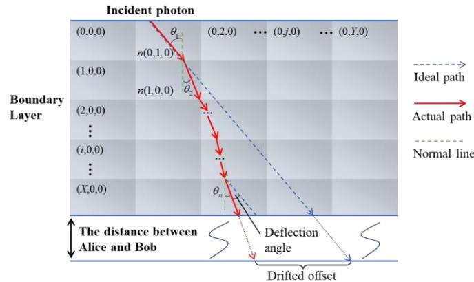
**Figure 2.** Two-dimensional schematic diagram of the ray tracing method.
