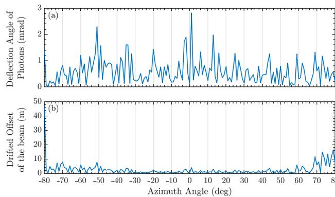
**Figure 5.** (a) The deflection angle of transmitted photons. (b) The drifted offset of the beam, which via the supersonic boundary layer and reaches the ground station.
