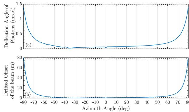
**Figure 4.** (a) The deflection angle of transmitted photons. (b) The drifted offset of the beam, which reaches to the ground station. The speed of airborne is 0.7 Ma.
