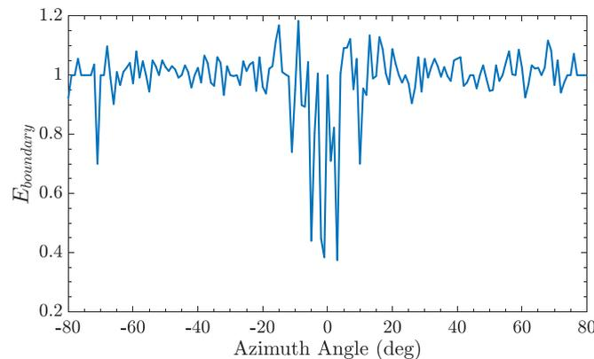
Figure 7. The receiving photons distribution probability ratio over the azimuth angle, when the photon via the supersonic BL.
