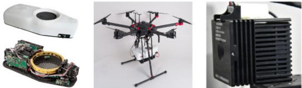
**Figure 1.** Airborne portable CH<sub>4</sub> laser spectrometer mainframe using a QCL (left), a spectrometer on-board system (middle) [32] and the wavelength of 8.9 μm and 3D dimensions of a 70 × 70 × 70 mm<sup>3</sup> micro QCL developed by our team (right).
