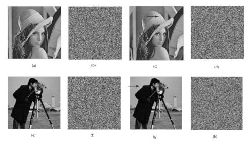
**Figure 18.** Comparison diagram before and after differential processing. (**a**,**e**) Plain-text image, (**b**,**f**) encrypted image, (**c**,**g**) plain-text image after differential processing, and (**d**,**h**) encrypted image after differential processing.
