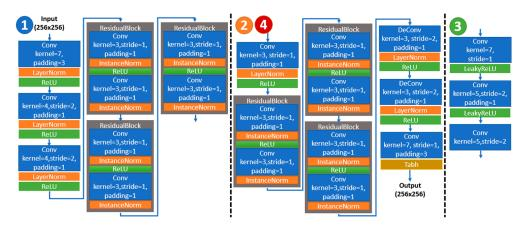
Figure 2. The layer structures of each subnetwork, indicated in Figure 1, for the proposed RD-Stego system.
