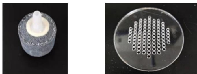
**Figure 15.** The air stone and the perforated circular plate.
