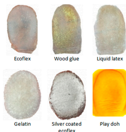
Figure 1. Examples of spoof artifacts fabricated using various commonly available materials [7].
