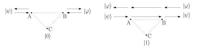
**Figure 4.** The examined entanglement level concerns mainly qubits *A* and *B*, which exchange their states (expressed as  $|\psi\rangle$  and  $|\varphi\rangle$ ) if controlling qubit  $C = |1\rangle$ . The entanglement level may also be analysed between pairs: *A*...*C* and *B*...*C*, which is marked above with the dotted line.
