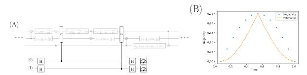
**Figure 8.** The scheme (**A**) of an exemplary quantum circuit estimating the entanglement level during switch's operating in a chosen point of the quantum circuit. The gates  $\pi_0$  and  $\pi_1$  realise the controlled SWAP operation. The chart (**B**) shows the entanglement values estimated by the circuit (as the difference of probabilities calculated for measuring state  $|0\rangle$  on both analysed qubits) and computed with the use of algebraic formula for the Negativity measure.
