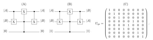
**Figure 2.** The circuits illustrating the operation of the quantum switch for qubits. If the state of the controlling qubit is  $|0\rangle$  (case (A)) the switch does not change the order of first two input states. When the state of the third qubit is expressed as  $|1\rangle$  (case (B)), the quantum switch swaps the input states  $|A\rangle$  and  $|B\rangle$ . The matrix (C) represents the unitary operator of the switch operation.
