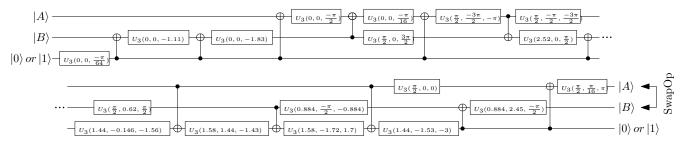
**Figure 3.** Decomposition of  $U_{qs}(t)$  operation for t = 1/4. The set of used gates enables the circuit's implementation in qiskit and quantum machine IBM Q. Decompositions may be realised for arbitrary *t* what requires the changes in values of rotating gates U3 parameters.
