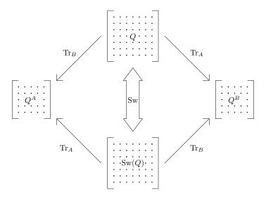
**Figure 1.** A graphical representation of the SWAP operation. Local information exchange is performed on the initial state Q (the final state, after the operation, is Sw(Q)). One can observe the swapping of subsystems A and B what may be calculated by the operation of partial trace.
