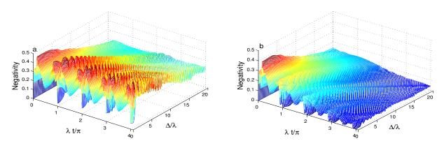
**Figure 6.** Entanglement dynamics for r = 0.5,  $\chi = 0$ ,  $|\zeta|^2 = 16$ ,  $\hat{Y}(\hat{\psi}^{\dagger}\hat{\psi}) = \sqrt{\hat{\psi}^{\dagger}\hat{\psi}}$  when the squeezed coherent state s = 0 with different qubit-cavity detuning values  $\Delta \in [0, 20]\lambda$ . We use  $\gamma = 0$  in (**a**) and  $\gamma = 0.1\lambda$  in (**b**).
