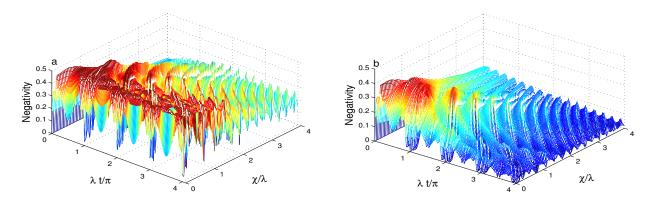
**Figure 7.** Entanglement dynamics for r = 0.5,  $\Delta = 0$ ,  $|\zeta|^2 = 16$ ,  $\hat{Y}(\hat{\psi}^{\dagger}\hat{\psi}) = \sqrt{\hat{\psi}^{\dagger}\hat{\psi}}$  when the squeezed coherent state s = 0 with different Kerr-like nonlinearity values  $\chi \in [0, 2]\lambda$ . We use  $\gamma = 0$  in (**a**) and  $\gamma = 0.1\lambda$  in (**b**).
