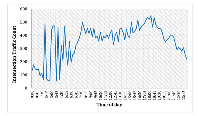
Figure 2. Atypical intersection count profile (severe fluctuations).
