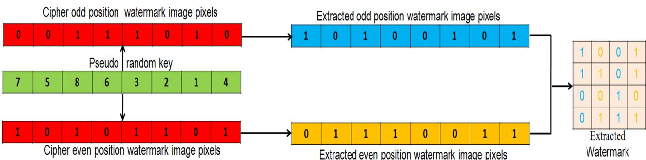
Figure 7. Watermark decryption at the receiver end.
