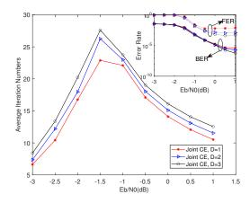
**Figure 7.** BER , FER, and convergence performance of joint CE in different depth factor at the same threshold factors when  $\alpha = \beta$ .
