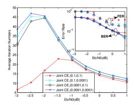
**Figure 6.** BER, FER, and convergence performance of joint CE in different threshold factors when one threshold factor is fixed and the other threshold factor is changed.
