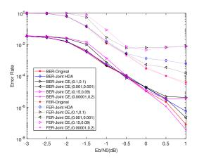
**Figure 8.** BER and FER performance of Original, joint HDA, and joint CE with different threshold factors.
