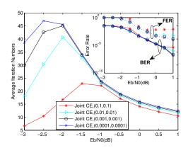
**Figure 5.** BER, FER, and convergence performance of joint CE in different threshold factors when  $\alpha = \beta$ .
