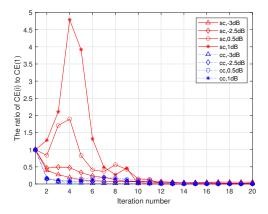
**Figure 4.** The ratio of cross entropy at the *i*-th iteration and cross entropy at the first iteration versus the decoding iteration numbers for the source decoder (solid curves) and channel decoder (dashed curves) at different  $E_h/N_0$ .
