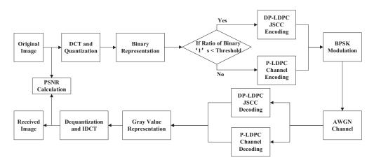
Figure 1. The image transmission system model.
