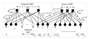
Figure 3. Joint decoder of the DP-LDPC system.
