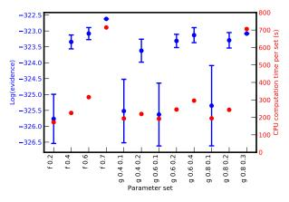
**Figure 7.** Values of  $\log E$  and CPU time for different choices of parameter values of the cluster recognition algorithm. Uncertainties of the evidence relative to the labels 'f 0.7' and 'g 0.8 0.3' are not evaluated because of the large computation time corresponding to these cases.
