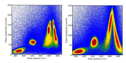
**Figure 5.** Joint probability distribution of the position and amplitude of one of the four considered peaks obtained without (**left**) and with cluster analysis (**right**).
