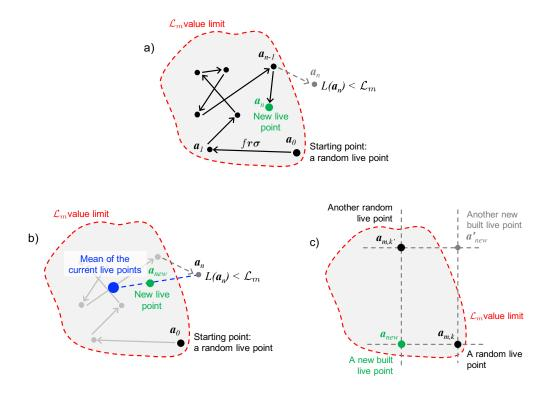
**Figure 1.** Graphical presentation of the different search algorithms discussed in the text. (**a**): Exploration of the parameter volume via the *lawn mower robot* for finding a new live point. (**b**): Search of a new live point from the parameter set  $a_n$  outside the limit  $L(a) > \mathcal{L}_m$  and the barycenter of the current live points. (**c**): Construction of the new live point from different coordinates of the current live points.
