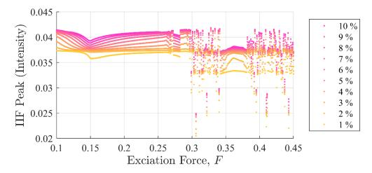
**Figure 15.** IIF peak values as a function of background excitation and discontinuity amplitude for case (ii). The separation in the discontinuity amplitude is apparent. The shape of the curves is very different from the global disturbance case due to the difference in sensitivity of the system to changes in stiffness. This was not the case for either SE or PEn.
