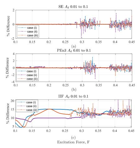
**Figure 17.** Difference values for cases (i), (ii), and (iii) as a function of excitation force. (a) SE results (b) PEn3 results (c) IIF results. The low values in (a) and (b) contrasted with the larger, consistently positive values in (c) show that the IIF is much better at distinguishing between the discontinuity levels.
