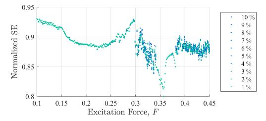
**Figure 5.** Shannon entropy values as a function of background excitation and discontinuity amplitude. The separation in the discontinuity amplitude test cases is not clear.
