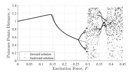
**Figure 1.** Poincaré distance showing the topological evolution of the Duffing oscillator with parameters:  $\zeta = .15, k = 1$ , and  $\Omega = 1.2$ . Forward and backward solutions are given in grey and black, respectively.
