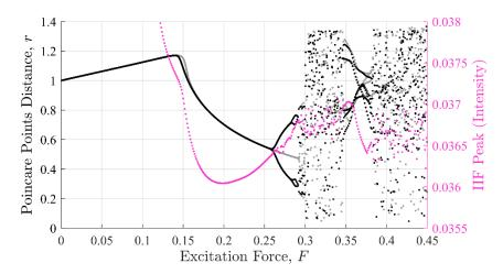
**Figure 10.** IIF peaks against the Poincaré distance. The shape the IIF peak values make as a function of excitation force mimics the Poincaré distance similarly to both the SE and PEn results, but with a smoother curve.
