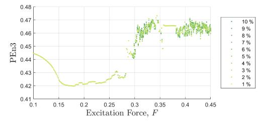
**Figure 6.** Permutation entropy values as a function of background excitation and discontinuity amplitude. There is no discernable separation in the discontinuity amplitude for most test cases.
