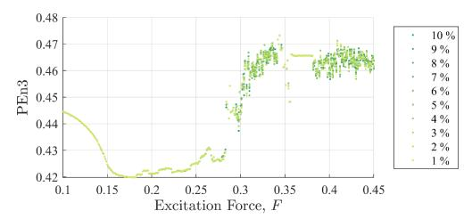
**Figure 12.** Permutation entropy values as a function of background excitation and discontinuity amplitude for case (ii). Like SE, these results closely follow those reported in Figure 7 for case (i).
