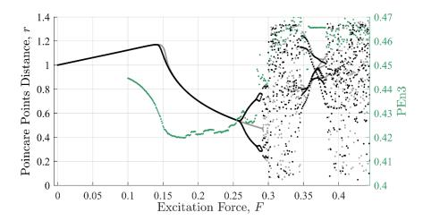
**Figure 9.** Permutation entropy against the Poincaré distance. The shape the PEn values make as a function of excitation force also mimics the Poincaré distance with similar inflection points. However, the shape loses form past F = 0.3.
