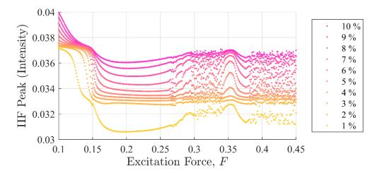
**Figure 7.** IIF peak values as a function of background excitation and discontinuity amplitude. Clear separation in the discontinuity amplitude test cases shows how well the IIF is able to detect a global disturbance even when the system is chaotic. The separation between amplitude test cases is in stark contrast to the SE and PEn results shown in Figures 5 and 6.
