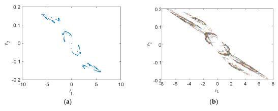
**Figure 5.** Poincaré maps on z = 0: (a) projection on the x–y plane, and (b) projection on the x–y plane with initial condition  $v_2(0)$  varying in the range of (-0.08, 0.08).
