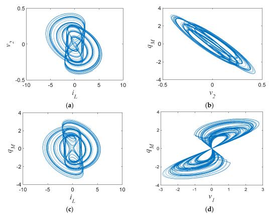
**Figure 4.** Chaotic attractors and chaotic  $v_1$ – $q_M$  hysteresis loops of the memcapacitor-based oscillator: (a–c) chaotic attractors; (d) chaotic  $v_1$ – $q_M$  hysteresis loops.
