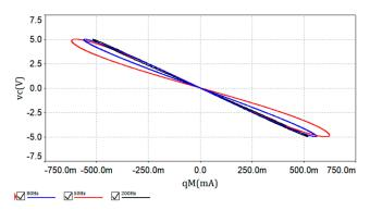
**Figure 2.**  $q_M$ – $v_C$  characteristic curves of the memcapacitor.
