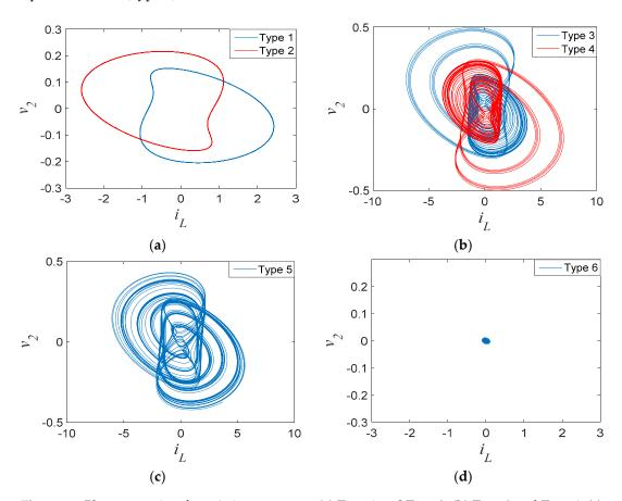
**Figure 11.** Phase portraits of coexisting attractors: (a) Type 1 and Type 2; (b) Type 3 and Type 4; (c) Type 5; (d) Type 6.
