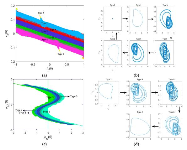
**Figure 12.** Basins of attraction of coexisting attractors in (**a**) the  $i_L(0)$ – $v_2(0)$  plane and (**c**) the  $q_M(0)$ – $\sigma_M(0)$  plane; the corresponding evolution process of coexisting attractors in (**b**)  $i_L(0)$ – $v_2(0)$  plane and (**d**) the  $q_M(0)$ – $\sigma_M(0)$  plane.
