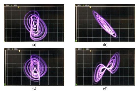
**Figure 15.** Chaotic attractors observed from the oscilloscope in the experiment: (**a**–**c**) chaotic attractors; and (**d**) chaotic  $v_1$ – $q_M$  hysteresis loops.
