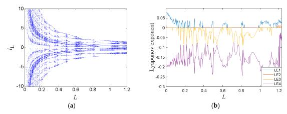
**Figure 6.** Dynamic characters with respect to *L*: (a) bifurcation diagram, and (b) lyapunov exponent spectrum.
