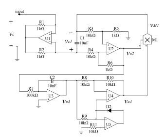
Figure 1. Equivalent circuit of the charge-controlled memcapacitor.
