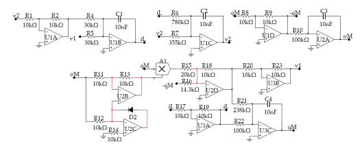
**Figure 13.** The equivalent circuit of the new system.
