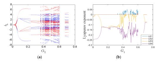
**Figure 7.** Dynamic characteristics due to  $G_1$ : (a) bifurcation diagram, and (b) Lyapunov exponent spectrum.
