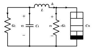
**Figure 3.** The memcapacitor-based chaotic oscillator.
