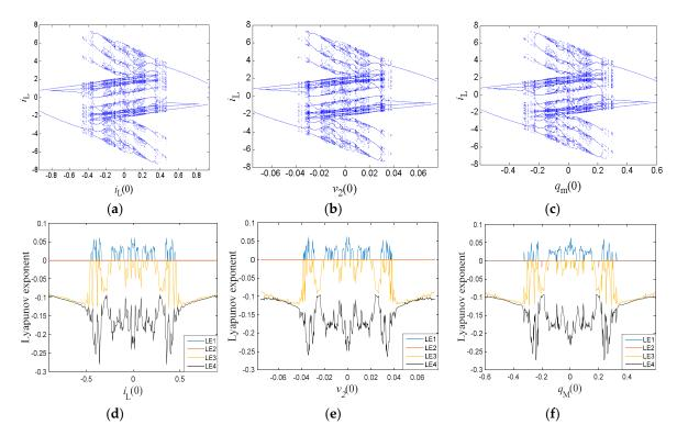
Figure 8. Dynamic characteristics: (a-c) bifurcation diagrams; and (d-f) Lyapunov exponent spectra.
