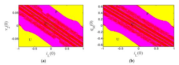
**Figure 9.** Dynamic maps of the system: (a)  $i_L(0)-v_2(0)$  plane, and (b)  $i_L(0)-q_M(0)$  plane.
