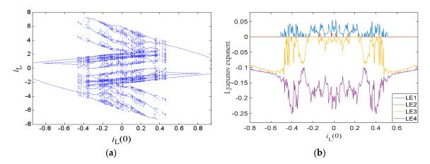
**Figure 10.** Dynamic characters due to  $i_L(0)$ : (a) bifurcation diagram, and (b) Lyapunov exponent spectrum.
