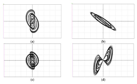
**Figure 14.** Chaotic attractors observed via Multisim simulations: (**a**–**c**) chaotic attractors; and (**d**) chaotic  $v_1$ – $q_M$  hysteresis loops.
