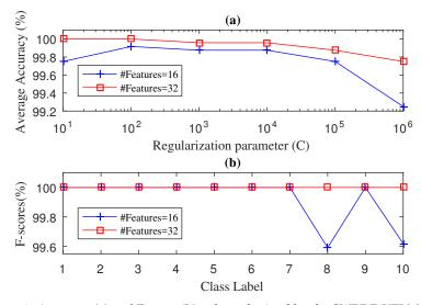
**Figure 5.** Diagnosis Accuracy (**a**) and F-score (**b**) values obtained by the SWPDE-KELM diagnosis with 5-Fold-CV during testing phase for fan-end bearing.
