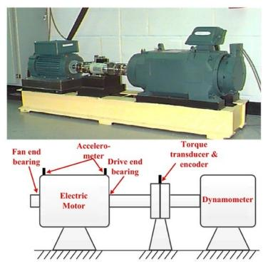
Figure 1. Experimental Setup [56].
