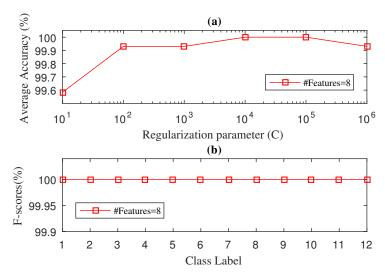
**Figure 2.** Diagnosis Accuracy (**a**) and F-score (**b**) values obtained by the SWPDE-KELM diagnosis with 5-Fold-CV during testing phase for drive end bearing.
