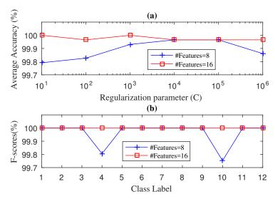
**Figure 3.** Diagnosis Accuracy (**a**) and F-score (**b**) values obtained by the SWPPE-KELM diagnosis with 5-Fold-CV during testing phase for drive end bearing.
