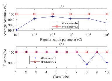
**Figure 6.** Diagnosis Accuracy (**a**) and F-score (**b**) values obtained by the SWPPE-KELM diagnosis with 5-Fold-CV during testing phase for fan-end bearing.
