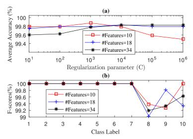
**Figure 7.** Diagnosis Accuracy (**a**) and F-score (**b**) values obtained by the SWPSVE-KELM diagnosis with 5-Fold-CV during testing phase for fan-end bearing.
