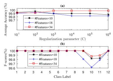
**Figure 4.** Diagnosis Accuracy (**a**) and F-score (**b**) values obtained by the SWPSVE-KELM diagnosis with 5-Fold-CV during testing phase for drive end bearing.
