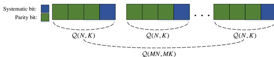
Figure 3. The codeword structure of quasi-uniform systematic polar code (QSPCs) with  $N = 4, K = 1$ .
