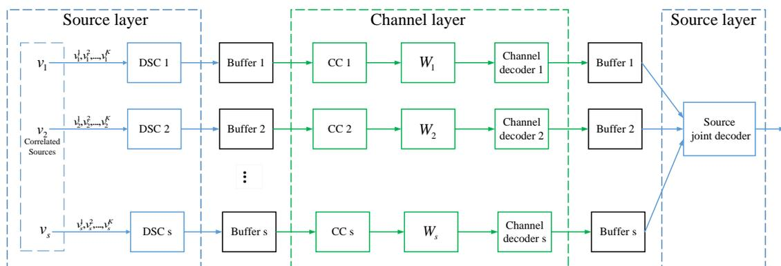
Figure 1. Distributed separate source-channel coding (DSSCC) scheme.
