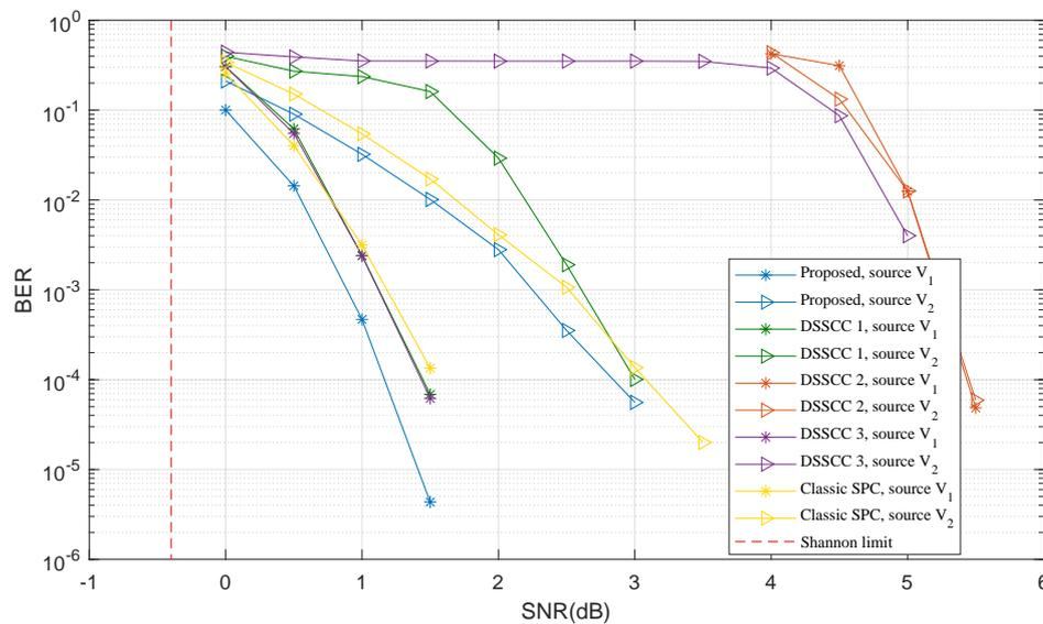
Figure 8. The BER performance under the CRC-aid SC list (CA-SCL) decoder.
