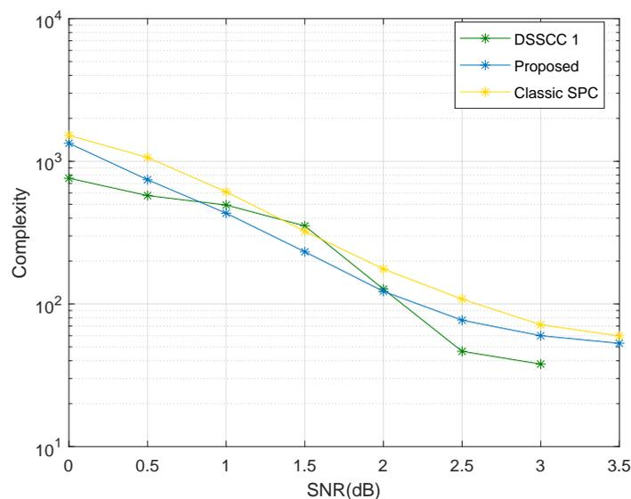
**Figure 9.** The decoding complexity (per source-symbol) under adaptive CA-SCL decoders.
