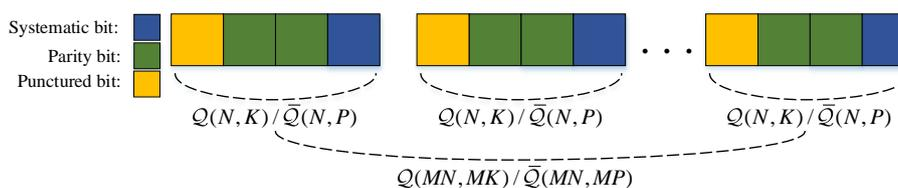
Figure 4. The codeword structure of punctured QSPCs with  $N = 4, K = 1, P = 1$ .
