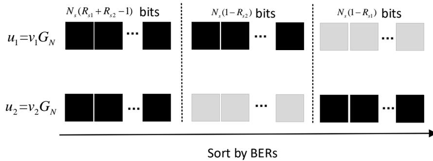
Figure 6. Bit selection of distributed source coding (DSC) based on polar codes.
