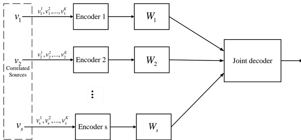
Figure 2. Distributed joint source-channel coding (DJSCC) scheme.
