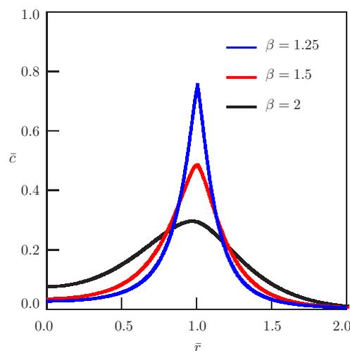
**Figure 6.** Dependence of the fundamental solution to the source problem on distance for  $\alpha = 0.5$ ,  $\bar{t} = 0.25$ ,  $\bar{b} = 0.5$  and various values of  $\beta$ .
