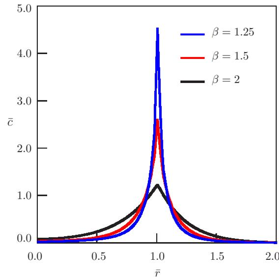
**Figure 4.** Dependence of the fundamental solution to the Cauchy problem on distance for  $\alpha = 0.5$ ,  $\bar{t} = 0.25$ ,  $\bar{b} = 0.5$  and various values of  $\beta$ .
