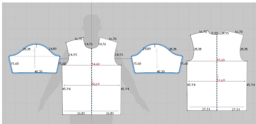
**Figure 4.** T-shirt pattern example. The highlighted measurements are the bust and waist girths of the T-shirt.
